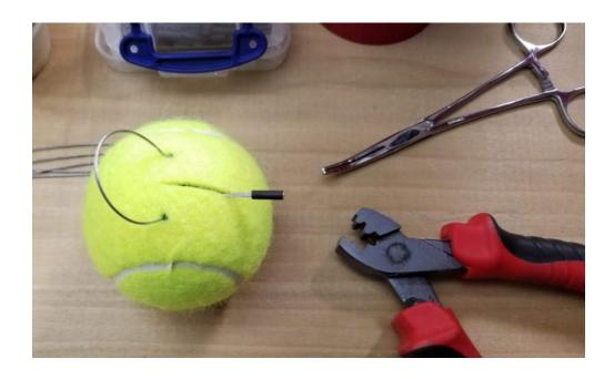
Slip the crimping tube on the wire ends and crimp the tube.
